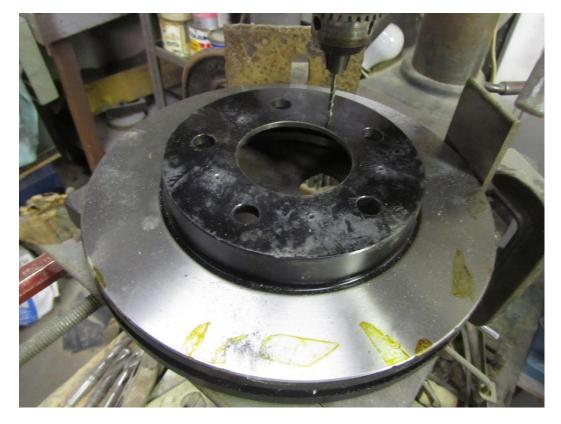
Holes are drilled using drills in the following diameter increments: 1/8", ¼", 3/8",7/16", ½" & 9/16". Notice that the finish hole size is oversized relative to the 7/16" wheel stud size. At 9/16" drill size the holes are similar to the factory wheel hole size. Factory tolerances allowed a wide variation between stud size and wheel hole size.
