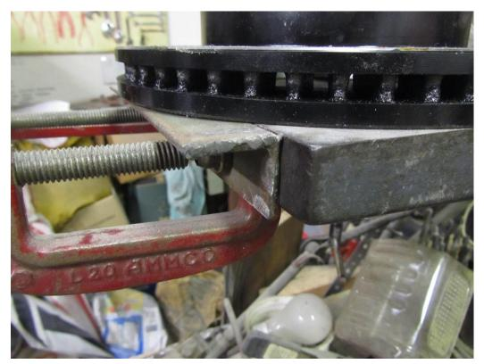
Location of these are done & adjusted until the rotor can be set up against the angles and each of the 5 holes aligned with the first step 1/8" drill. The disc rotor is rotated several times & each hole checked to insure angles are properly located:
