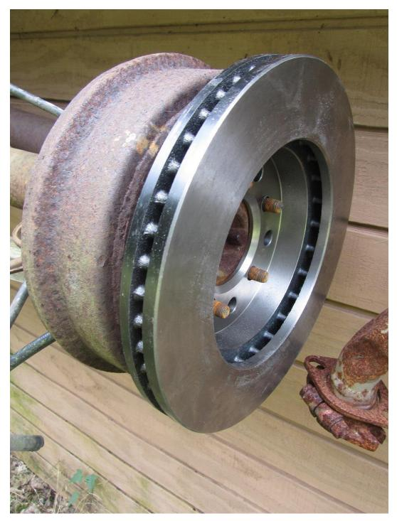
The above fitting was done on a rear axle since the hub drill pattern and centering hub are the best for using as a guide for determining accuracy of the hole spacing.
